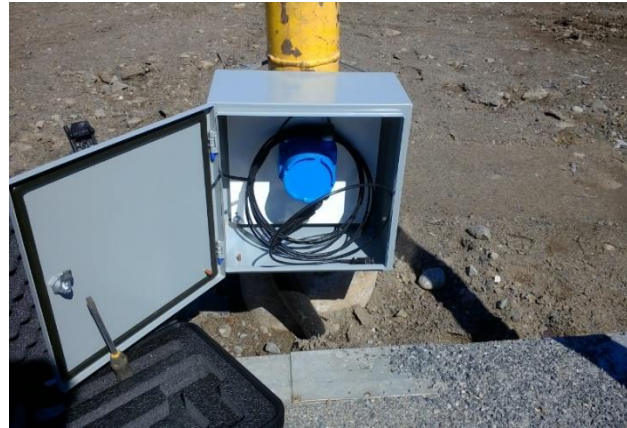
smartPIMS or matPIMS collection point resides inside box for periodic data collection
