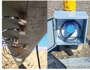
Buried probes attached to pipe and connected to a smartPIMS® Modbus DSI in an above-ground enclosure.
